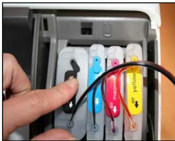
Slightly press every cartridge to check all the cartridges are in the correct position. Please be careful with the tubes which go out from Cartridge Carrier. Then stick the Support Arm on the position which shown in the third picture.
