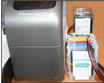
Put the CISS on the left side of the printer. In the meantime place all the tubes at correct position.
