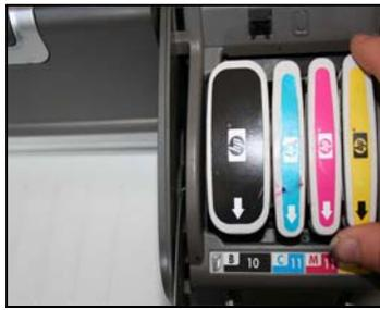
Remove the original cartridges
