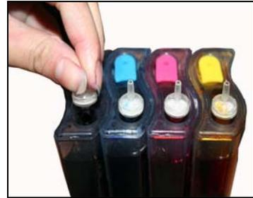
Place 4pcs of air filters into air holes, the thicker side is down into tank.
